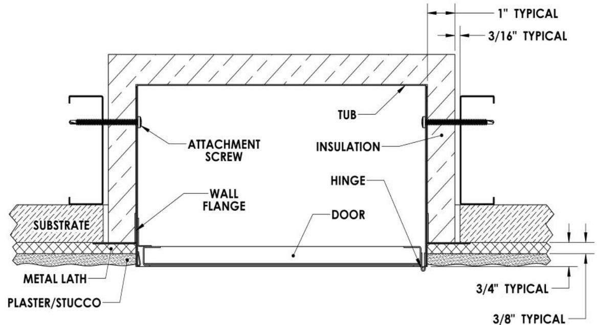
Note: Drawings shown on this page are examples only of typical installation in a fire-rated wall, and are not to be used as recommendations for wall construction.
