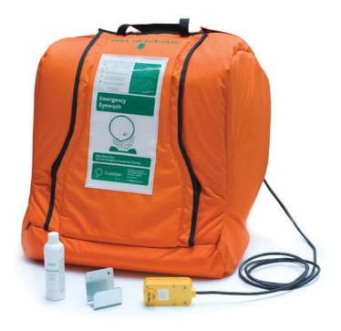
**Preparation:** To operate unit, fill with clean potable water and add bacteriostatic additive (supplied with unit). Additive protects against growth of bacteria, fungus, algae and acanthamoeba. Unit should be inspected regularly and water should be changed at least once every six months.
