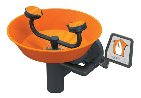
**Application:** Eye/face wash for wall mounting. Constructed entirely in PVC and PVC-coated brass. Ideal for use in industrial environments where harsh acids or caustics are present. Two large FS-Plus<sup>™</sup> spray-type outlet heads deliver a flood of water for rinsing eyes and face.
