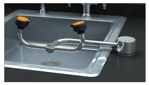
**Application:** AutoFlow™ eyewash for mounting on counter next to sink. Swinging the spray head assembly 90 degrees horizontally out over the sink activates the water flow. The unit remains in operation until the spray head assembly is swung back into the storage position, closing the valve.
