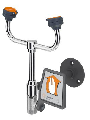
**Application:** Eyewash for wall mounting. Two GS-Plus<sup>™</sup> spray-type outlet heads deliver a flood of water for rinsing eyes. Unit is provided without bowl or drain for waste water. Note: Floor drain should be provided underneath unit to prevent accumulation of water on floor.
