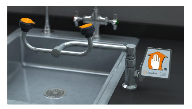
**Application:** All-stainless steel eyewash for mounting on counter next to sink. Spray heads swivel 90 degrees from storage to operational position. Unit is constructed entirely in stainless steel. Ideal for use in highly corrosive environments, cleanrooms and pharmaceutical applications.
