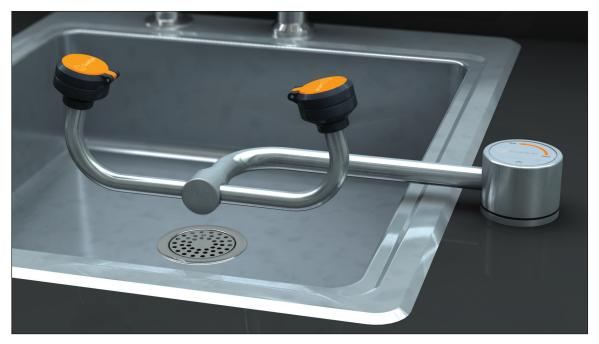
**Application:** All-stainless steel AutoFlow™ eyewash for mounting next to sink. Unit is constructed entirely in stainless steel. Ideal for use in highly corrosive environments, cleanrooms and pharmaceutical applications. Swinging the spray head assembly horizontally out over the sink activates the water flow. The unit remains in operation until the spray head assembly is swung back into the storage position, closing
