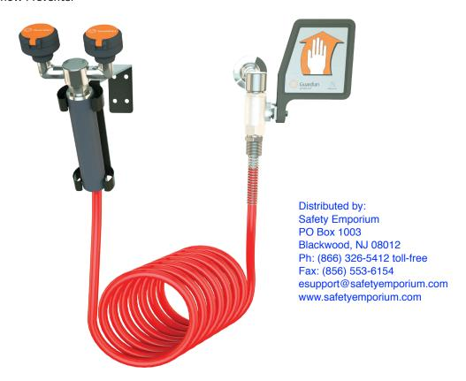
**Application:** Dual purpose eyewash/drench hose with ball valve and flag handle for wall mounting. Unit meets the provisions of ANSI Z358.1-2014 as both an eyewash and a drench hose. Unit may be left in the mounting bracket for use as a fixed eyewash, leaving user's hands free. Alternatively, unit may be removed for use as a drench hose to rinse any part of user's eyes, face or body. 12' nylon retractable hose coils to eliminate trip hazard.
