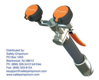
**Application:** Dual purpose eyewash/drench hose unit for 45 degree angled panel mounting. Unit meets the provisions of ANSI Z358.1 -2014 as both an eyewash and a drench hose. Unit may be left in the angle holder for use as a fixed eyewash, leaving user's hands free. Alternatively, unit may be removed for use as a drench hose to rinse any part of user's eyes, face or body.
