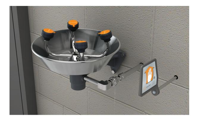
**Application:** Freeze-resistant WideArea<sup>™</sup> eye/face wash for wall mounting. Valve and supply line are located behind wall in heated area to prevent freezing. Self-draining valve permits water to drain completely from unit after use. Since unit is intended for use in cold weather conditions, consideration should be given to supplying unit with tempered water in accordance with ANSI Z358.1-2014. See "Tempering Units" section for more information.
