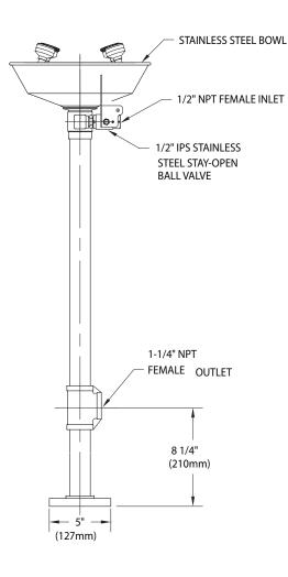
EACH GS-PLUS SPRAY HEAD HAS A "FLIP-TOP" DUST COVER, INTERNAL FLOW CONTROL AND FILTER TO REMOVE IMPURITIES FROM THE WATER FLOW.
