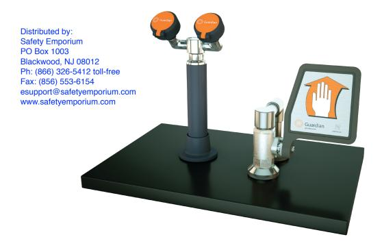
**Application:** Dual purpose eyewash/drench hose with ball valve and flag handle for deck mounting. Unit meets the provisions of ANSI Z358.1-2014 as both an eyewash and a drench hose. Unit may be left in the deck flange for use as a fixed eyewash, leaving user's hands free. Alternatively, unit may be removed for use as a drench hose to rinse any part of user's eyes, face or body.
