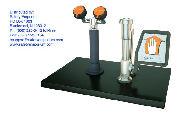
**Application:** Dual purpose eyewash/drench hose with ball valve and flag handle for deck mounting. Unit meets the provisions of ANSI Z358.1-2014 as both an eyewash and a drench hose. Unit may be left in the deck flange for use as a fixed eyewash, leaving user's hands free. Alternatively, unit may be removed for use as a drench hose to rinse any part of user's eyes, face or body. Vacuum breaker prevents external water and contaminants from seeping back into supply line.
