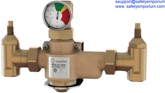
**Application:** Thermostatic mixing valve to blend hot and cold water to deliver tepid water. Valve has flow capacity of 50 gallons (189 liters) per minute at 30 PSI (2.1 bar) pressure drop. Valve can be used to supply emergency shower or combination safety station. Depending on water supply size and pressure, valve can supply multiple units.
