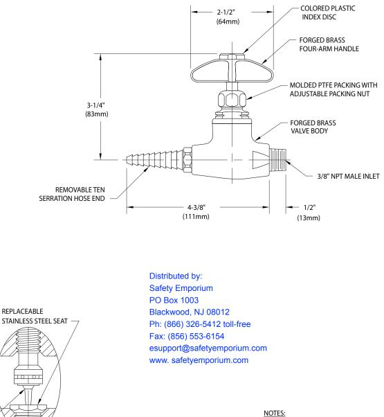
REPLACEABLE FINE METERING STAINLESS STEEL FLOATING NEEDLE
