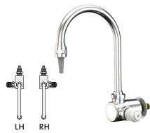
**Application:** Panel mounted faucet for distilled, deionized or reverse osmosis water. Faucet has exterior brass casing and interior lining of inert polypropylene. Pure water comes in contact only with inert plastic.
