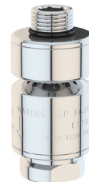
L110: Dual check vacuum breaker. ASSE-certified under Standard 1035. 3/8" NPS male inlet, 3/8" NPT female outlet.
