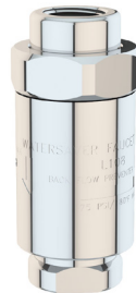
L108: Dual check backflow preventer. For continuous pressure applications. ASSE-certified under Standard 1024. 3/8" NPT female inlet and outlet.
