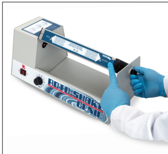
4. Depress and hold the Release button, slide Lock Shaft into Platform through the housing. Hand-tighten Lock Shaft fully into place then let go of the Release button
