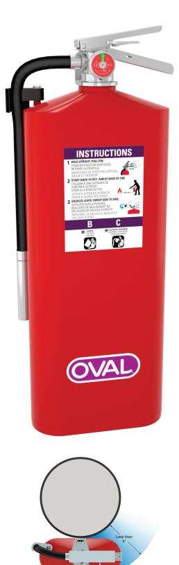
**Application:** 10 lb. Purple K dry chemical fire extinguisher for wall and column mounting. Highly effective on flammable liquid fires. Suitable for use on Class B and C fires. Not recommended for use on sensitive electronic equipment.
